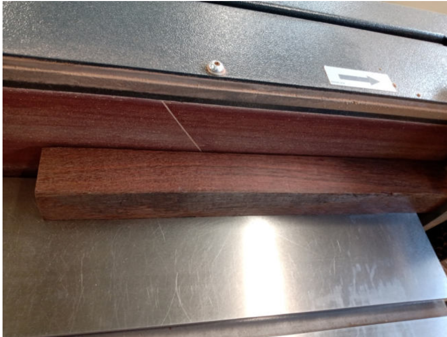
Figure 3, please note timber against the stop and trailing edge making contact first
