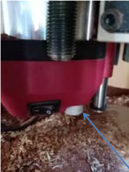
Picture 5, speed adjustment control knob
